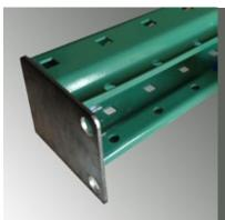
Our patent pending no-weld base plate that looks and acts like a welded plate has a simple 3 part construction (welded nut, washer & bolt) for quick and easy assembly. Dimples in the plate lock the baseplate and columns into position, further easing assembly (base plate can be welded if desired).
